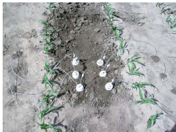
Figure 4 - Pore water sampling at different depths in an agriculture soil
