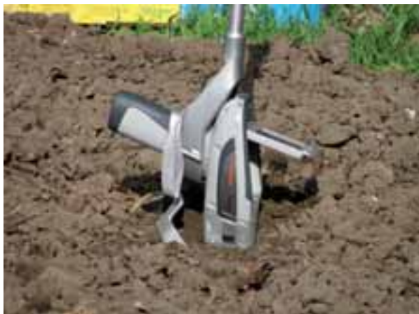
Fig. 4. Field-portable x-ray fluorescence spectrophotometer sampling for preliminary total soil trace element concentrations.
