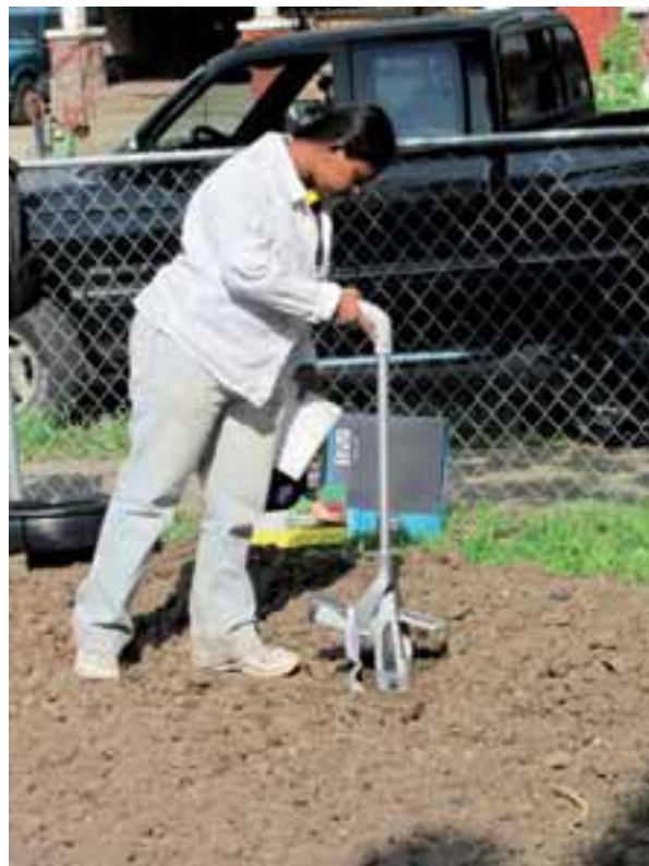
Fig. 5. Conducting preliminary soil tests for total soil trace element concentrations on the Michigan Avenue vacant lot using the field-portable x-ray fluorescence (XRF) spectrophotometer. A handheld GPS was used to record the position of the XRF measurement, and a field notebook was used to record the GPS waypoint and the XRF sampling point number. The data is downloaded from both devices and merged in a spreadsheet.
